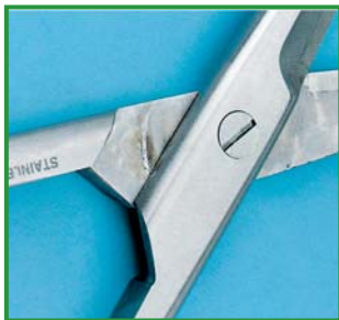
Fretting corrosion due to inadequate lubrication
