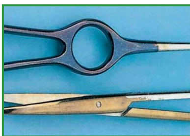
Instruments discoloured by silicic acid
