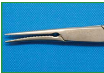
Deformation caused by improper handling
