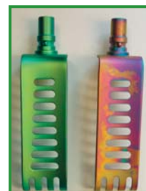
Left valve: brand new - uniformly green Right valve: machine-cleaned - strongly discolored
