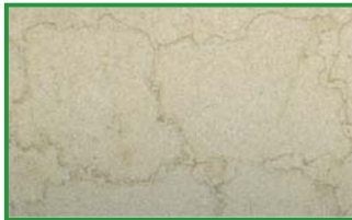
Marbling caused by impurities in steam condensate
