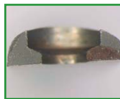
Breakage at countersunk screwhead
