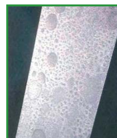
Instrument surface with drip-like discoloration
