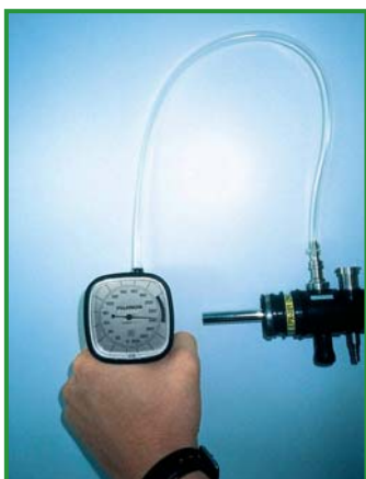
Manual leakage test on flexible endoscope
