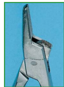
Jaw breakage on suture holder
