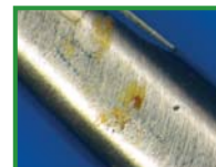
Microscopically magnified (200x) corrosion hole
