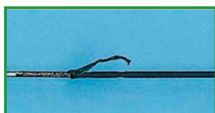
Damaged insulation on HF instrument
