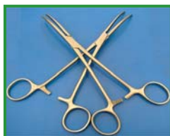
Contact corrosion between two instruments both made of stainless steel
