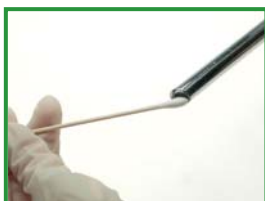
Cleaning the lens of an endoscope
