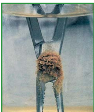
Corrosion caused by immersion in physiological salt solution over a period of several hours
