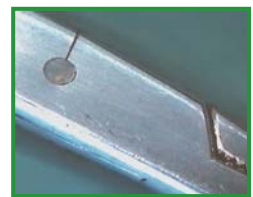
Fracture at hinge pin
