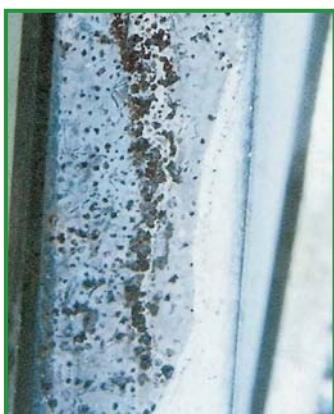
Deposits on instrument formed by substance containing chloride
